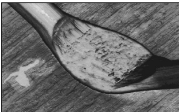
Figure 1. Ultrasonic Wire Bonded Joint. 0.001" aluminum wire bonded to ½ ounce electrodeposited copper on RT/duroid 6010. No attempt to clean the copper foil surface was made, but the result is still a good joint.
