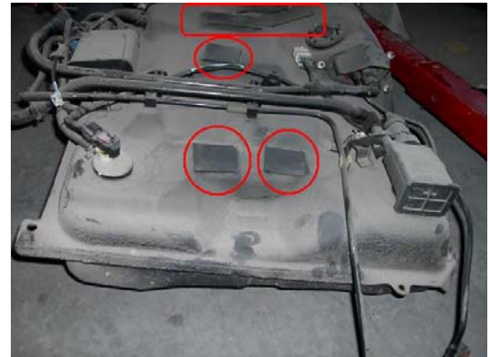
Automotive Fuel Tank with PORON Isolator Pads Circled
